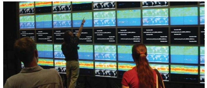
Collaboration and concurrent visualization of 20 simulation runs performed by the International Panel on Climate Change (IPCC). The Highly Interactive Parallelized Display Wall (HIPerWall) project provides unprecedented high-capacity visualization capabilities to experimental and theoretical researchers. Credit: Falko Kuester, California Institute for Telecommunications and Information Technology, University of California-San Diego
