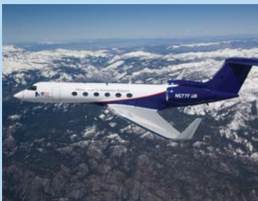
HIAPER (High-Performance Instrumented Airborne Platform for Environmental Research) aircraft in flight. HIAPER, modified Gulfstream V jet, can fly at an altitude of 51,000 feet and has a range of 7,000 miles. The aircraft’s range enables scientists to survey remote ocean regions in a single flight to learn more about interactions between the oceans and the atmosphere. Credit: © University Corporation for Atmospheric Research
